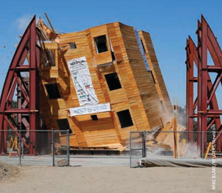
A four-story wood frame building is tested under the conditions of a number of historical earthquake data using the world's largest outdoor shake table by researchers at the University of California San Diego. Tangshan, China: A partial view of Tangshan City in Hobei province where an earthquake with a force of 7.8 on the Richter scale rocked the city on July 28, 1976.
